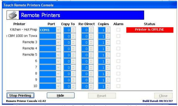
This screen is remote printer 1 (the first line) has the name kitchen Hot prep and is located on com 1 of this till, the status is currently offline as it is out of paper or the printer switched off
